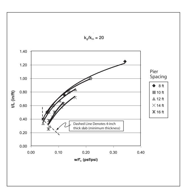
Figure 6. Normalized Thickness Required for Stiffness Ratio ( $\rm k_g$  / $\rm k_m$ ) of 20
