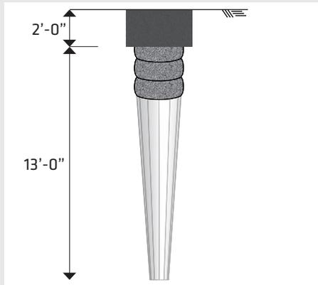
The non-production RAP used for modulus testing was installed through soft clay and loose sand. Deflection measurements were taken during the modulus test. A two foot thick concrete cap was poured over the top of the RAP for testing purposes.
