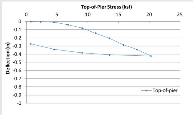
The results of the modulus test indicate that a deflection of 0.20 inches was observed at the maximum top-of-RAP design stress of 13,500 psf, with corresponding RAP stiffness modulus at 469 pci.
