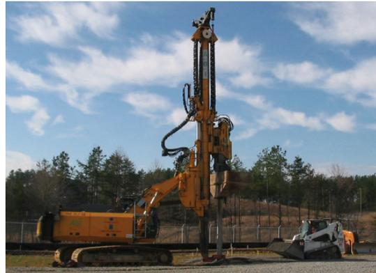
28 feet to reinforce the soils. Modulus testing confirmed the RAP design with less than 0.5 inches of deflection at a top-of-pier stress level of greater than 21 ksf.
