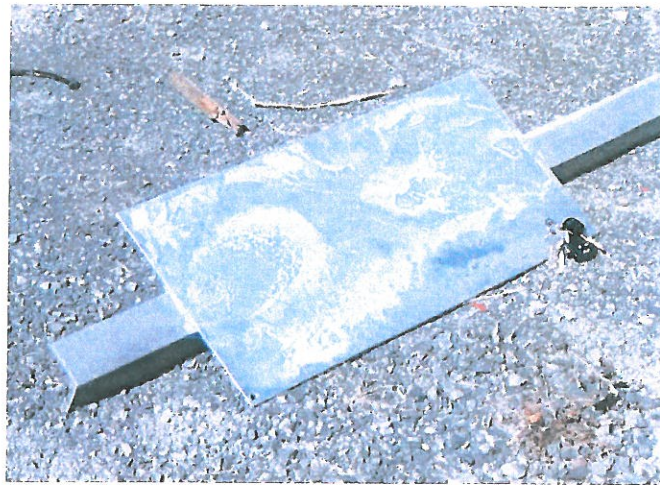
FIGURE 3 Details of typical galvanized steel plate pile.
