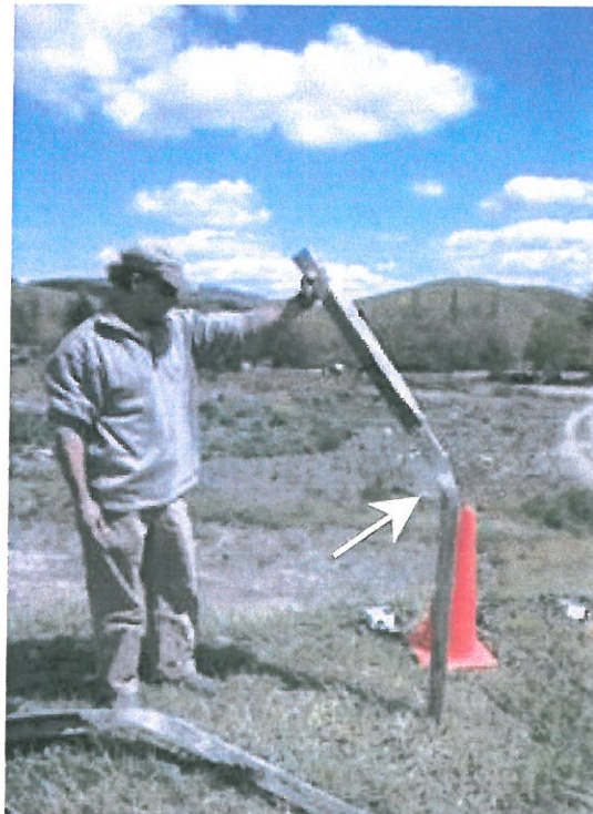
FIGURE 9 Ultimate strength testing of plate piles with formation of hinge point at yield.
