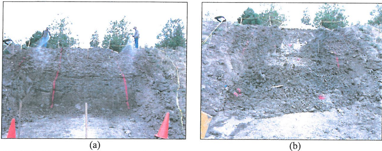
FIGURE 7 Test 1 -without plate piles (a) during irrigation and (b) following failure.
