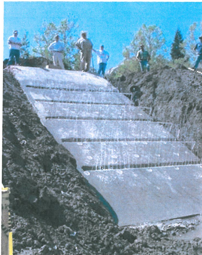
FIGURE 5 The Blackhawk GHAD Test Site with bottom irrigation tubes turned on.
