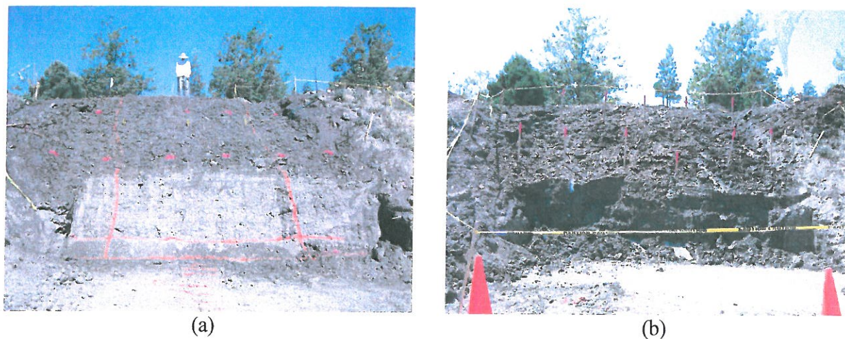
FIGURE 8 Test 2 - with plate piles (a) during irrigation and (b) at end of test without failure.
