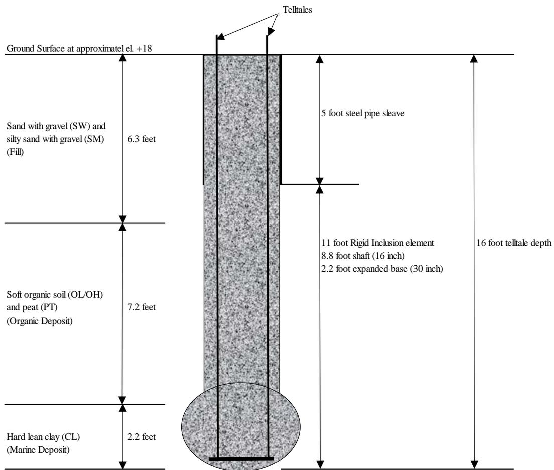
Figure 5: Stand-Alone Test Element
