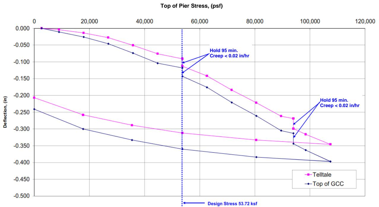
**Figure 6: Stand-Alone Load Test Results**
