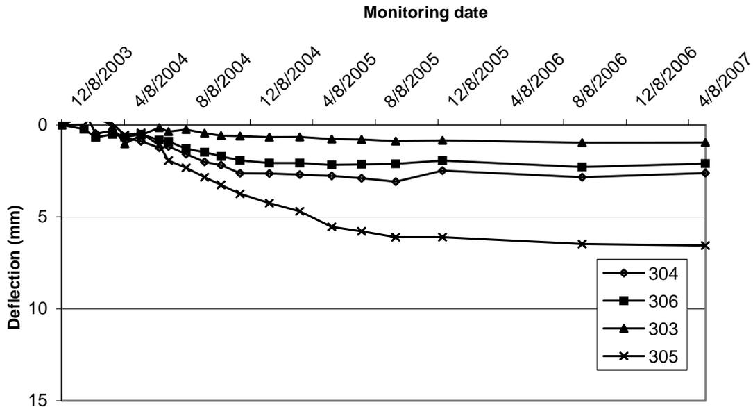
Figure 8. Compression of the reinforced zone vs. monitoring date
