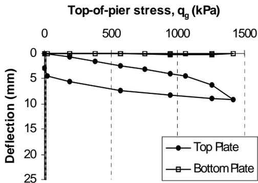
Figure 5. Modulus test results of test pier A
