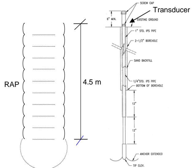
Figure 7. Extensometer schematic
