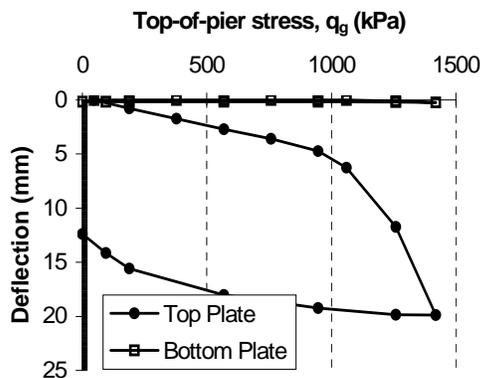
Figure 6. Modulus test results of test pier B
