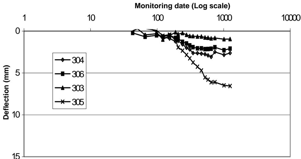
Figure 9. Compression of the reinforced zone vs. days of monitoring (log scale)
