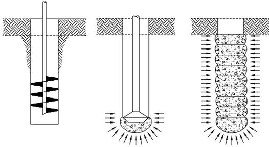
Figure 3. Geopier Rammed Aggregate Pier Construction
