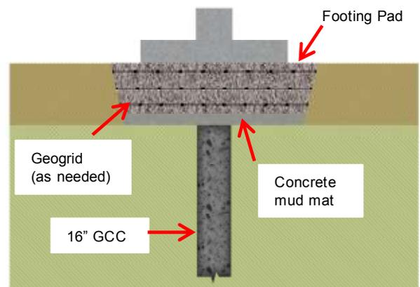
Figure 6 – Footing Pad Detail
