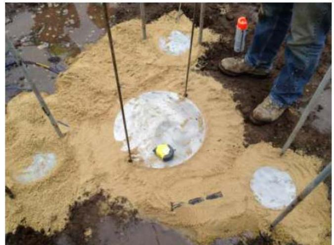
Figure 10 – Pressure Cells Bedded in Sand
