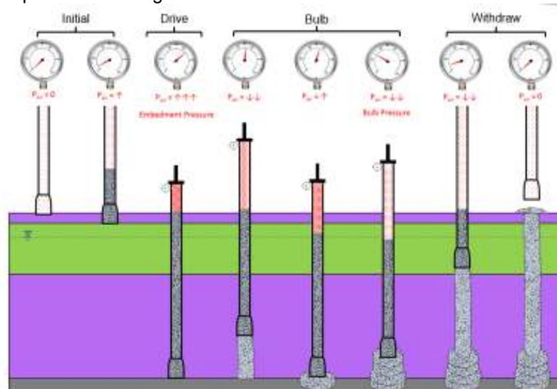
Figure 8: GCC construction sequence, indicating air pressure and volume relationship with each stage of pier construction
