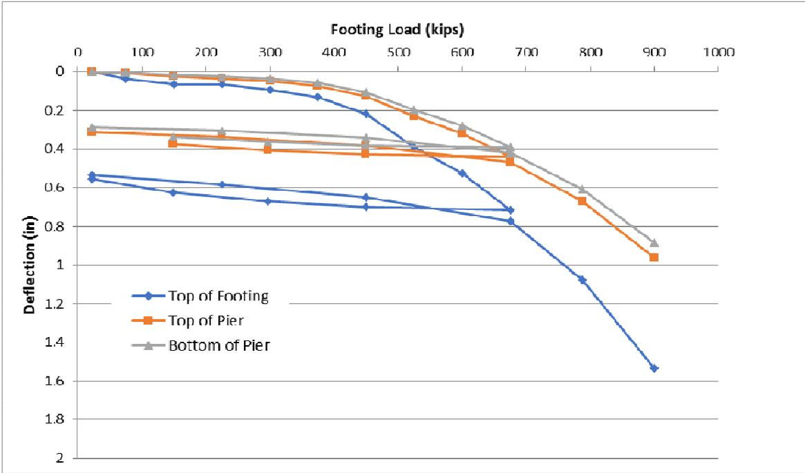
Figure 11 – Load Test Results - Measured Deflections
