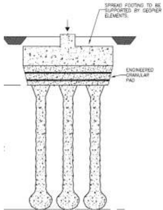
Figure 4: Typical Footing Detail
