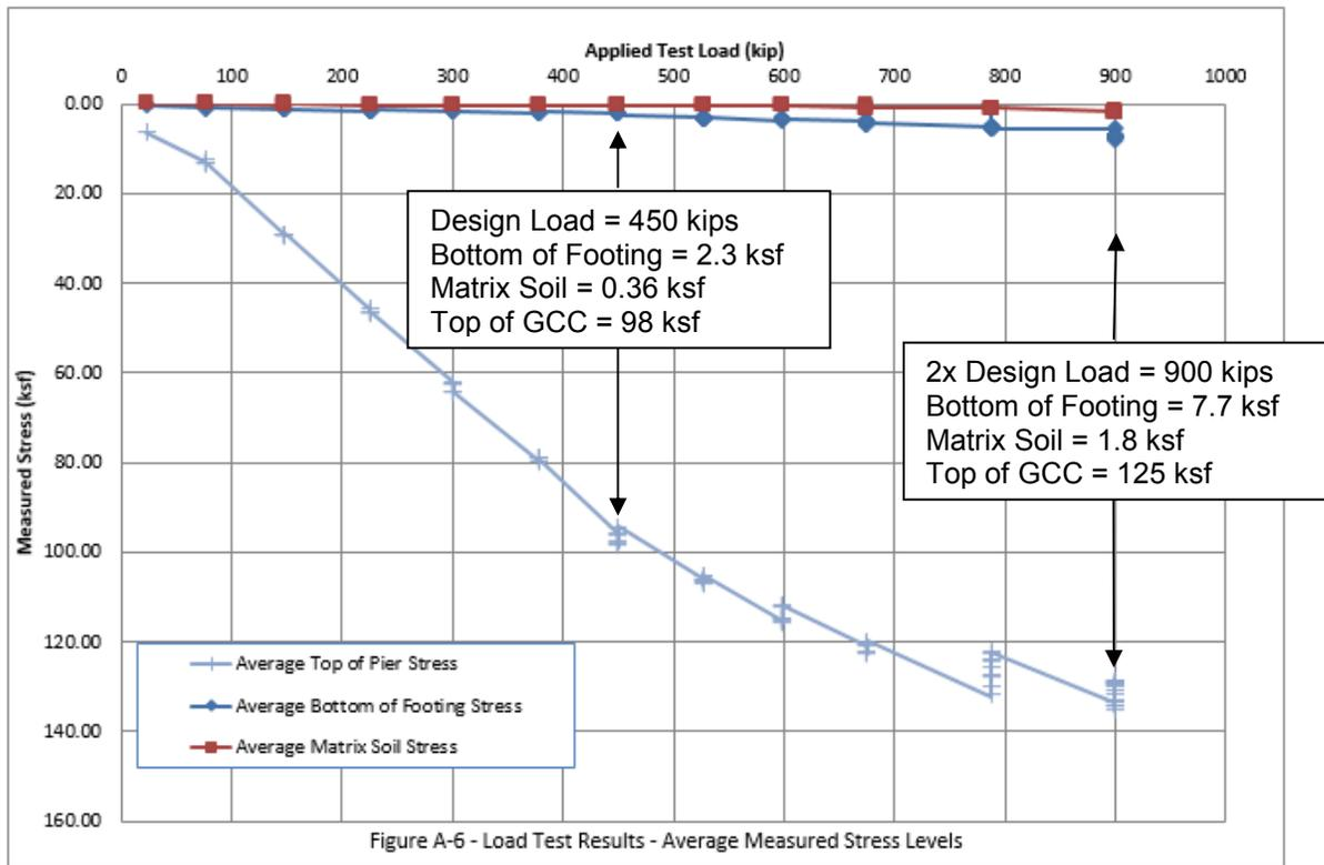
Figure 12 – Load Test Results – Averaged Measured Stress Levels
