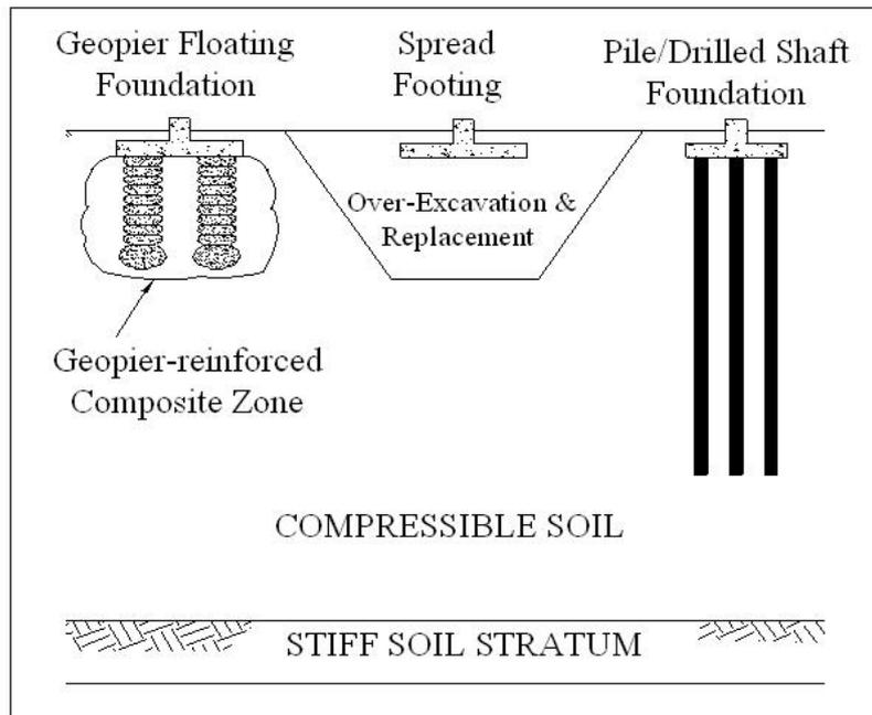
Fig. 1 Concept of floating foundations
