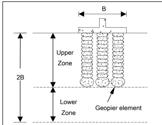
Fig. 7 Schematic of upper- and lower-zone
