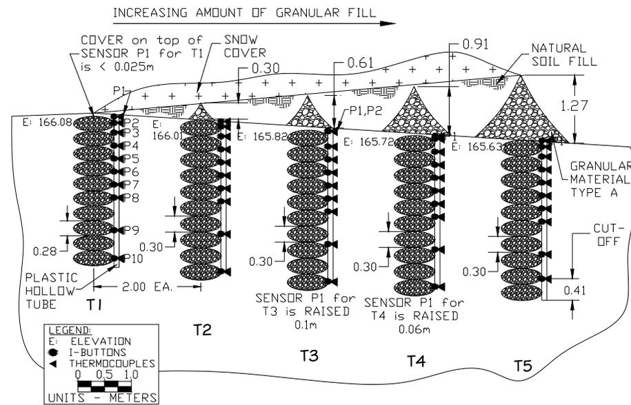
Figure 3. Pier profile layout
