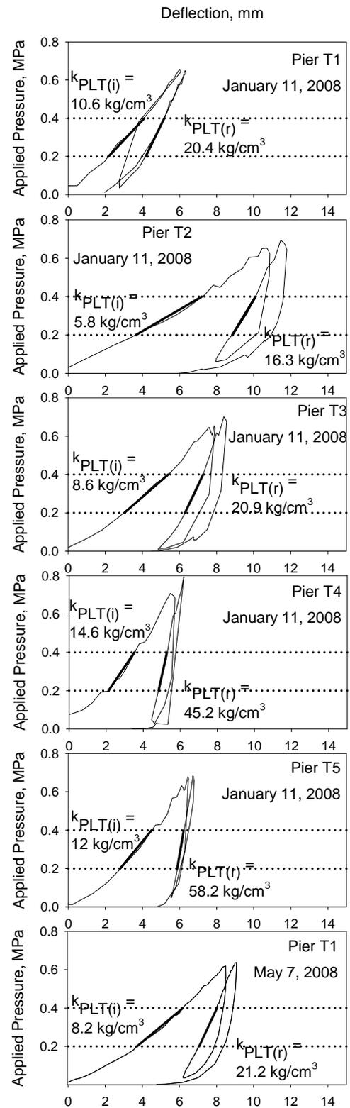
Figure 12. Stress-strain curves from 300 mm plate diameter static plate load tests ( $k_{PLT(i)}$  – initial stiffness and  $k_{PLT(r)}$  – reload stiffness)
