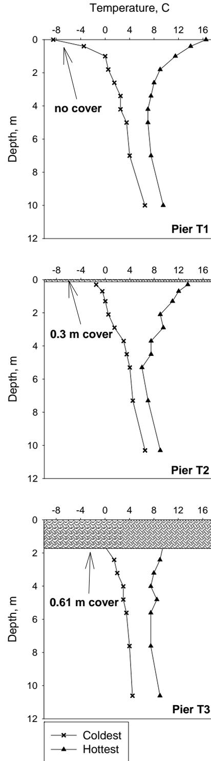
Figure 10. Extreme temperature profiles for piers T1, T2, T3 – coldest to warmest recorded
