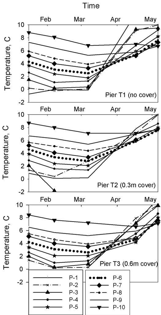
Figure 6. Thermocouple temperature sensor records for piers T1, T2, T3
