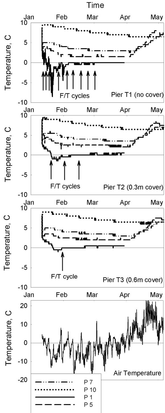
Figure 8. I-Button temperature sensor records for piers T1, T2, T3 and air temperature
