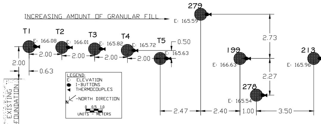
Figure 2. Pier plan layout
