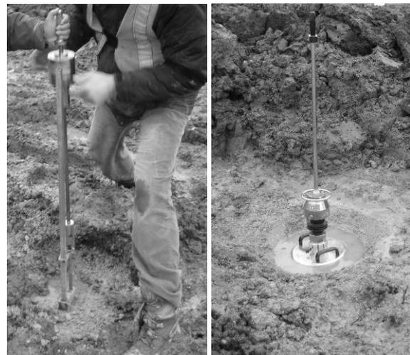
Figure 5. Dynamic cone penetrometer test (left), (b) Light weight deflectometer test (right)
