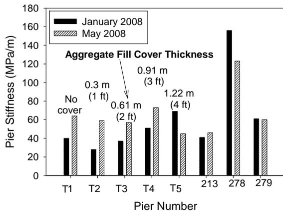
Figure 13. Comparison of  $E_{iwd}$  stiffness values before and after winter (soil cover information provided for T1 – T5, unknown for piers 213, 278, and 279)
