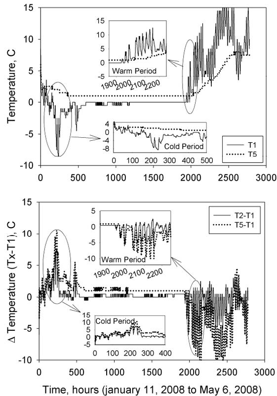
Figure 9. Comparison between top of pier temperatures during measurement period (top), and difference between test piers with cover and test pier T1 with no cover (+ indicates insulation) (bottom)
