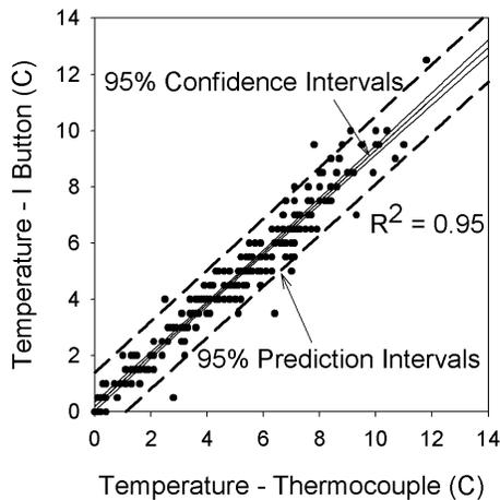
Figure 7. Thermocouple versus I-Button temperature correlation
