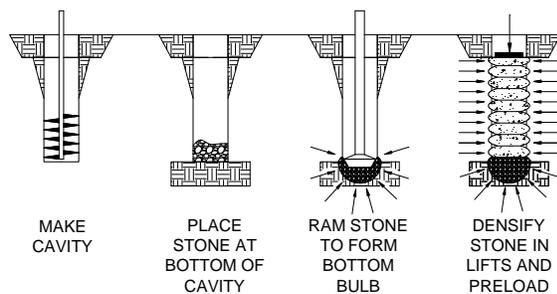
Figure 1. Simplified pier installation process
