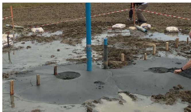
Fig. 9. Multiple sand boils and ejecta, the evidence of liquefaction, observed during Blast 1 near the center of the unimproved natural panel (NP). (Image by Kyle M. Rollins.)
