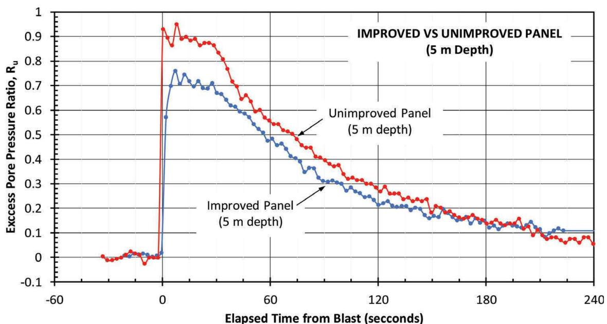
Figure 5. Comparison of preliminary measured excess pore pressure vs. time curves for improved and unimproved panels at a depth of 5 m below the ground surface.
