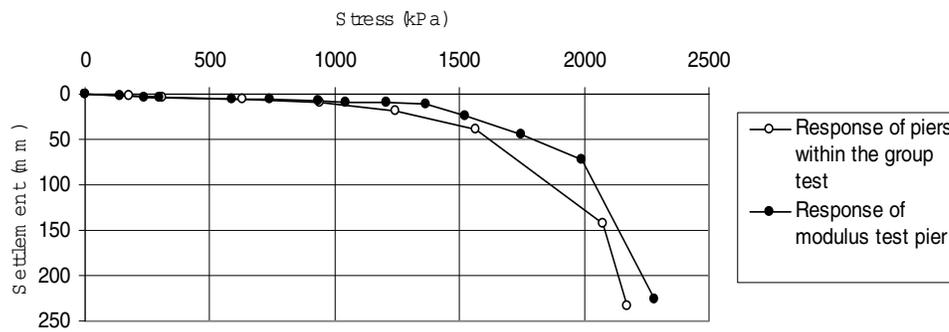
**Figure 6: Utah modulus test vs group test comparison**
