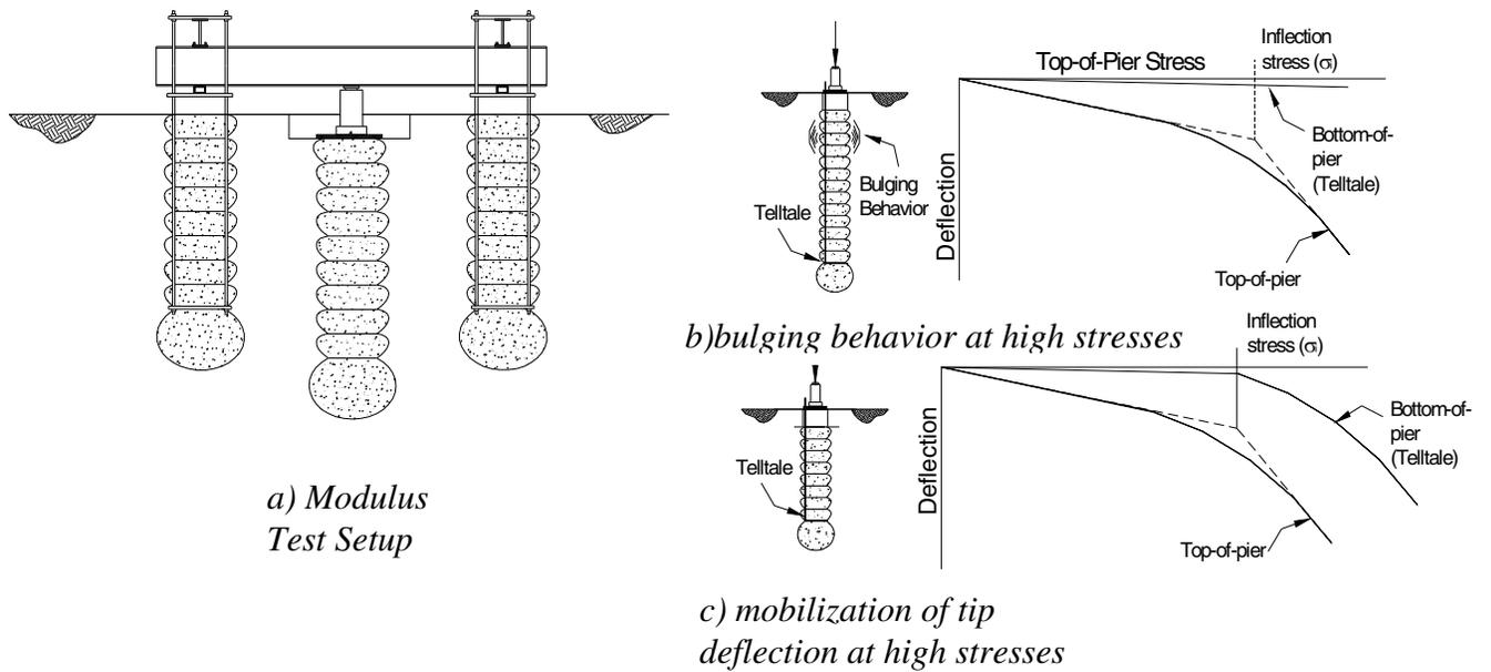
**Figure 3: Modulus test results and interpretation**
