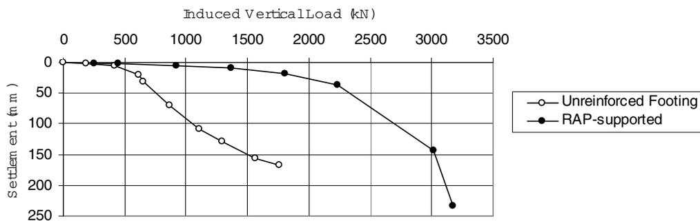
**Figure 7: Utah group load test comparisons**
