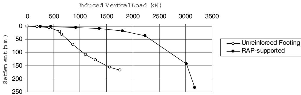
**Figure 7: Utah group load test comparisons**
