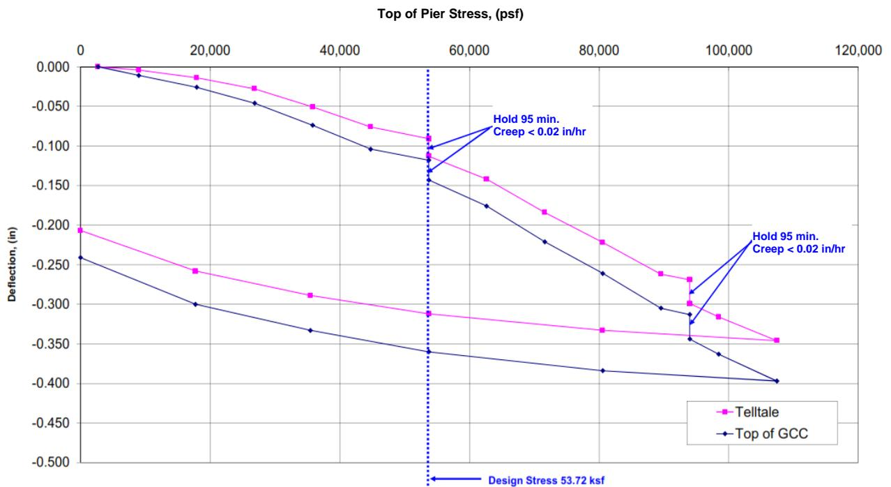
**Figure 6: Stand-Alone Load Test Results**
