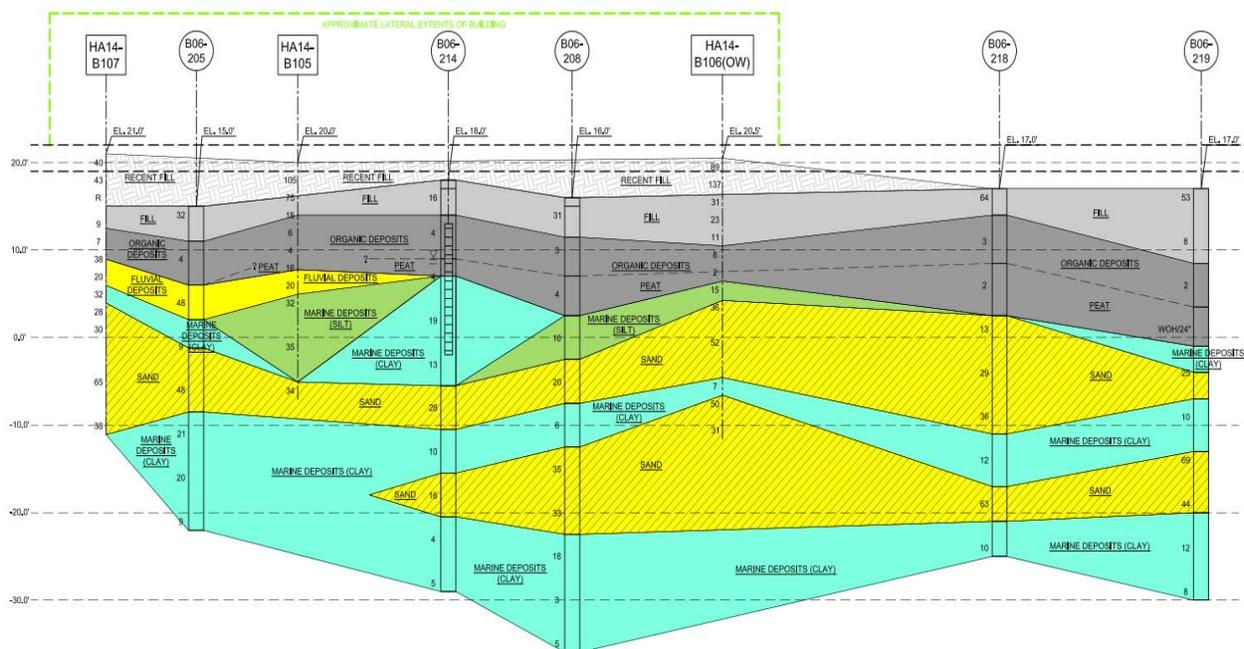
**Figure 2: Typical Subsurface Profile (Figure created by Haley & Aldrich)**
