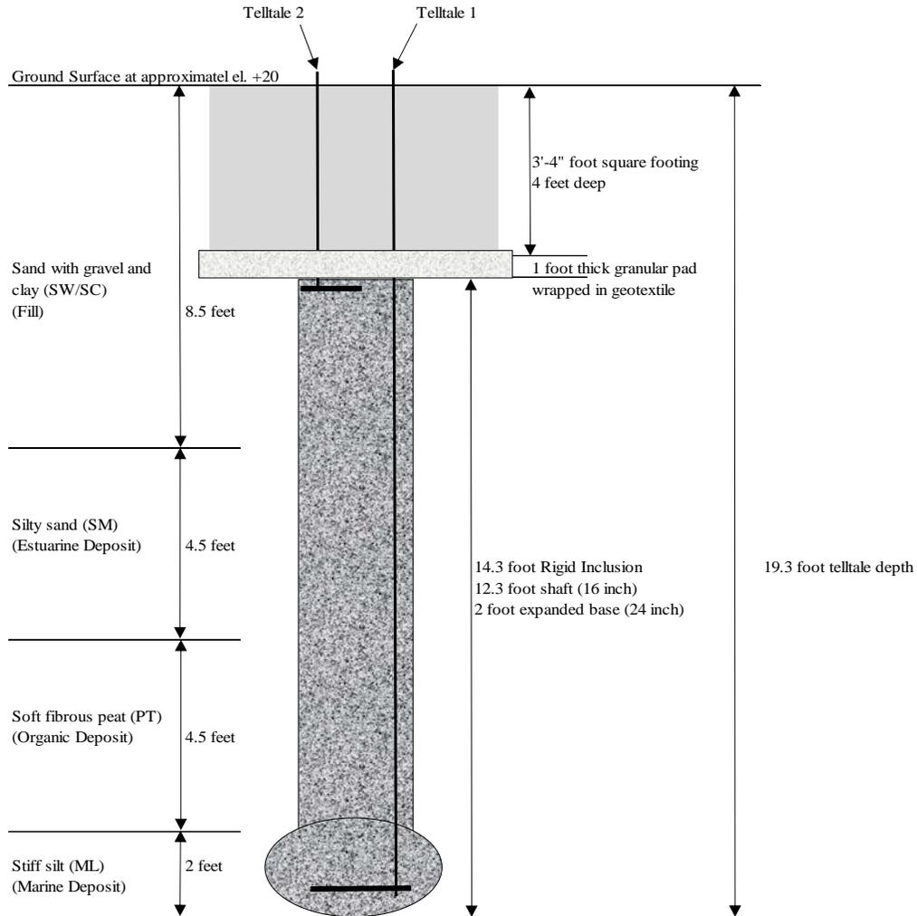
**Figure 7: Test with Granular Pad and Footing**
