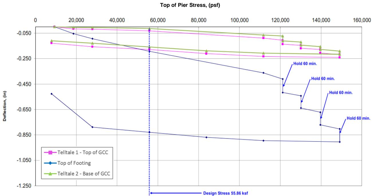
**Figure 8: Granular Pad and Footing Load Test Results**
