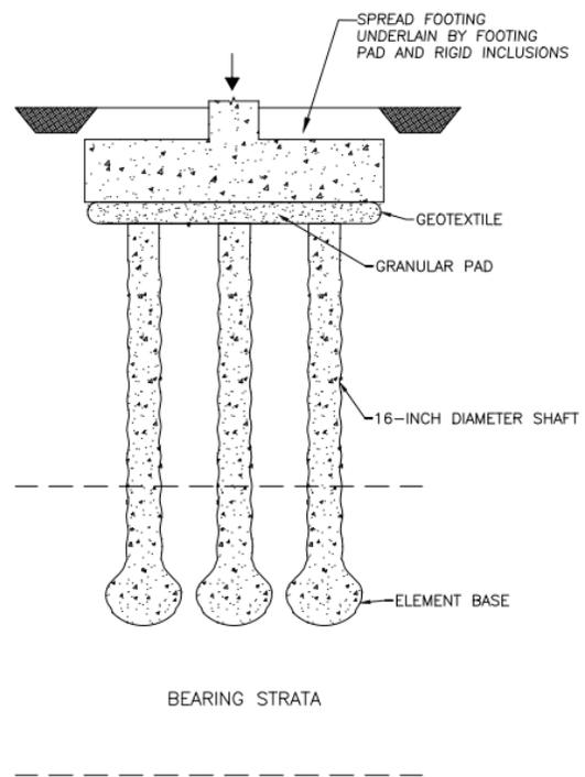
**Figure 3: Typical System Configuration**
