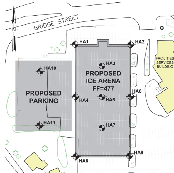
Figure 2 - Subsurface Exploration Program
