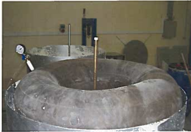
Figure 2. A large size inner tube used as an airbag placed in the tank to apply pressure
