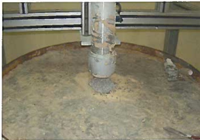
Figure 3. View of the tank following the installation of rammed aggregate piers
