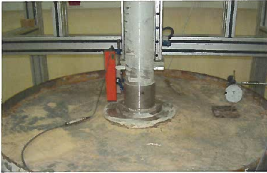
Figure 4. Location of plate and displacement measurements for plate loading test
