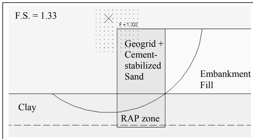
**FIG 5: Stability output for Rammed Aggregate Pier-reinforced soil**
