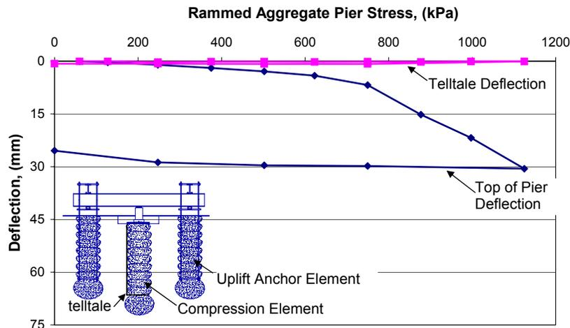
**FIG 8: Rammed Aggregate Pier Modulus test results**
