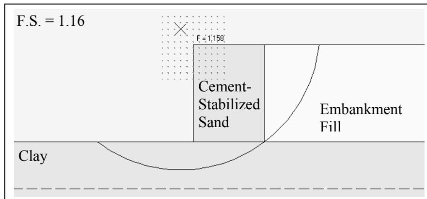
**FIG 3: Stability output for MSE wall on unreinforced foundation**
