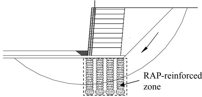
**FIG 4: Rammed aggregate pier support of MSE wall**
