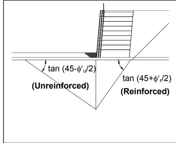
**FIG 7: Rankine's lower-bound bearing capacity solution**
