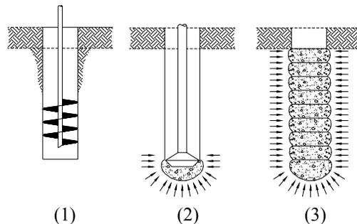
**FIG 2: Rammed aggregate pier construction process**
