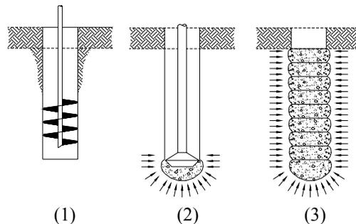
**FIG 2: Rammed aggregate pier construction process**
