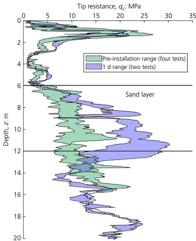
Figure 8. Range of pre-installation CPTs (CPT-1, -2, -3 and -4) compared to the range of CPTs conducted 1 d after installation (CPT-5 and -6)
