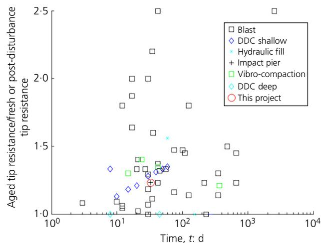
**Figure 14.** Ageing effects compared to disturbance method highlighting the data from this project, the first documented case of sand ageing following impact rammed aggregate pier installation
