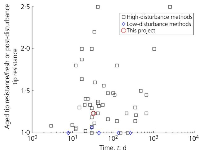
**Figure 15.** Ageing effects compared to high-disturbance and low-disturbance methods highlighting the data from this project.
