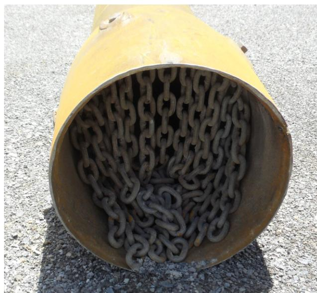
Figure 1. Proprietary 'Impact Pier' mandrel used in installation of displacement rammed aggregate piers
