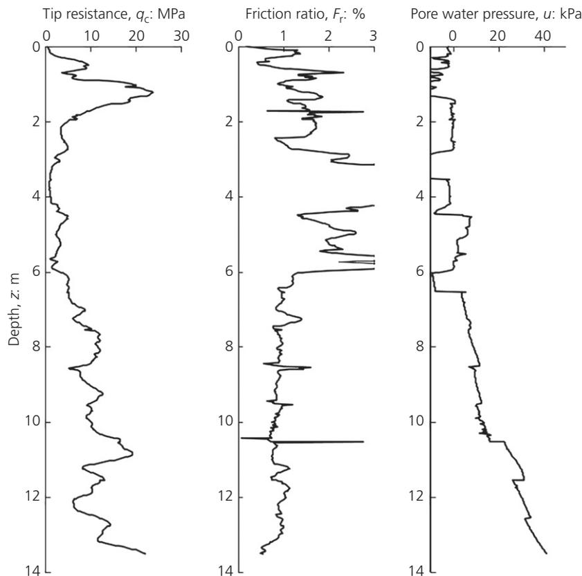
Figure 5. Results from CPT-4, typical of pre-installation testing.  $F_r$  greater than 3% is not shown for clarity
