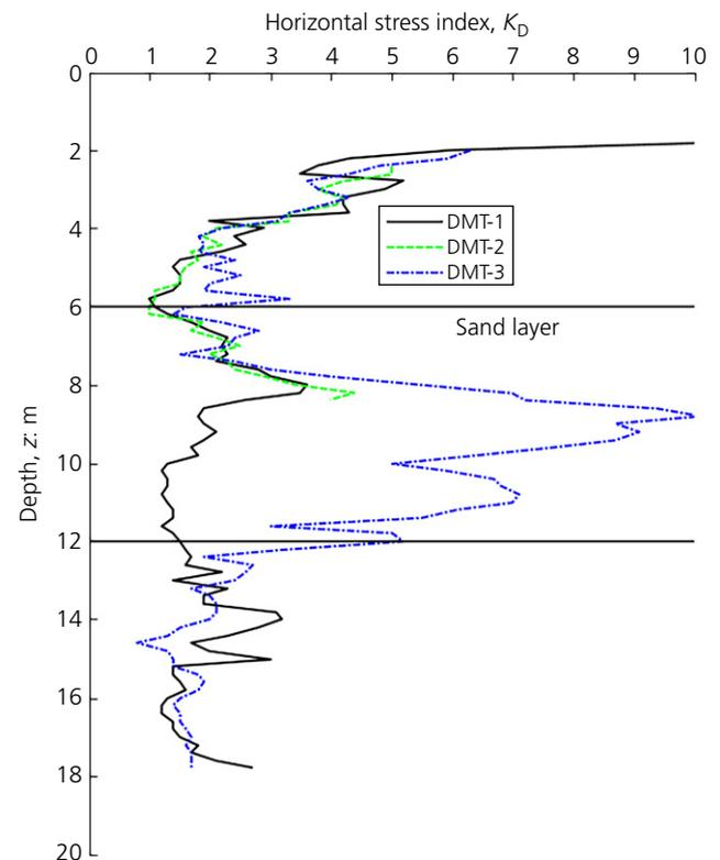
Figure 9. DMT horizontal stress index from DMT-1 conducted before installation and tests conducted 1 d after installation (DMT-2 and -3)
