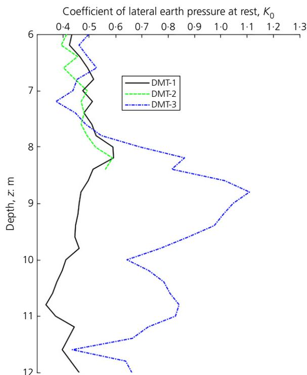
Figure 11. Coefficient of lateral earth pressure at rest as determined from DMT-1 conducted before installation and tests conducted 1 d after installation (DMT-2 and -3)
