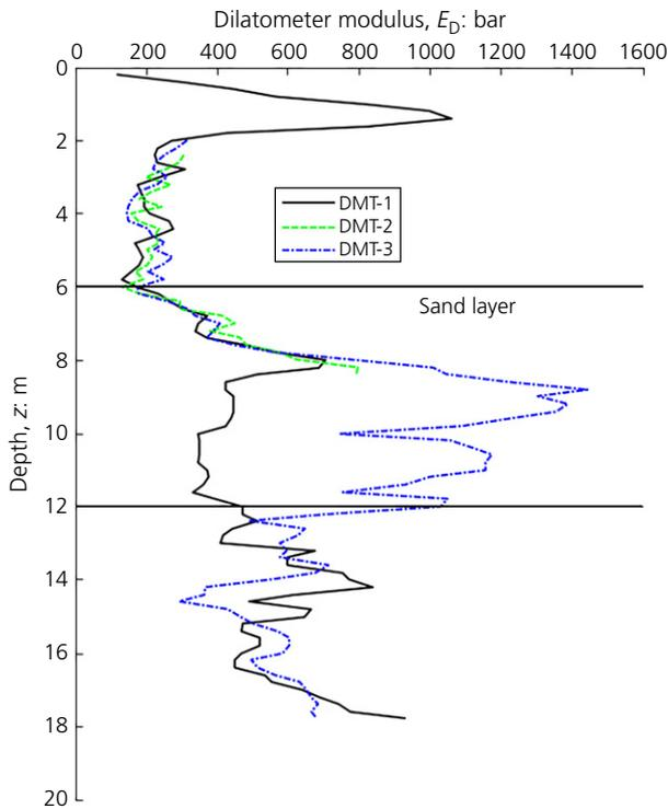
Figure 10. Dilatometer modulus from DMT-1 conducted before installation and tests conducted 1 d after installation (DMT-2 and -3)
