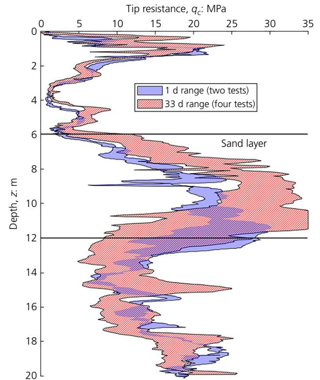
Figure 12. Range of  $q_c$  from CPT conducted 1 d after installation (CPT-5 and -6) compared to range of  $q_c$  from CPT conducted 1 month after installation (CPT-200, -201, -202 and -203)
