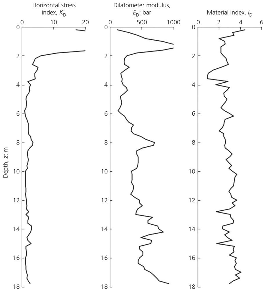
Figure 7. Results of DMT-1, conducted prior to pier installation.  $K_D$  and  $E_D$  greater than 20 and 1000 bars, respectively, are not shown for clarity
