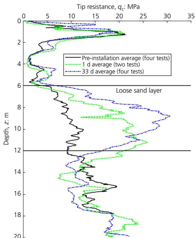
**Figure 13.** Mean CPT  $q_c$  from testing before, within 24 h and 1 month following pier installation
