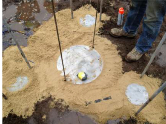
Figure 9: (a) Rigid inclusion test layout; (b) Test instrumentation showing telltales and total stress pressure plates.
