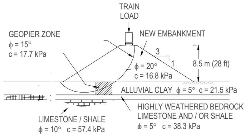
**Figure 7: Iowa railroad embankment stability results**
