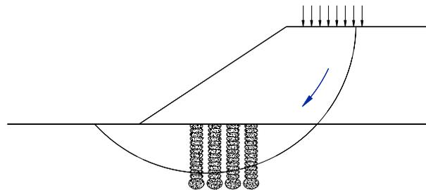
**Figure 4: Global stabilization using Geopier elements**
