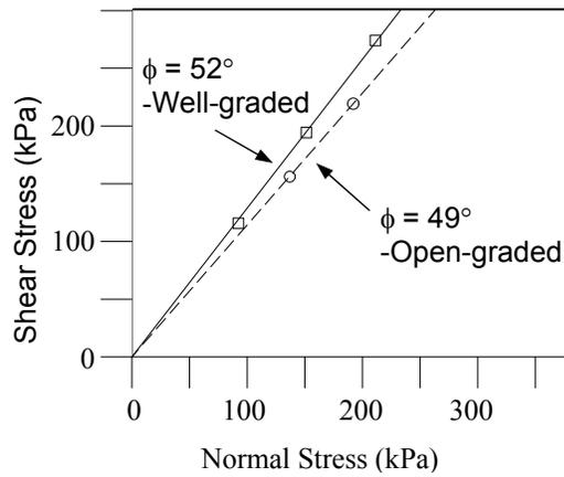
**Figure 3: Results of full-scale direct shear tests**
