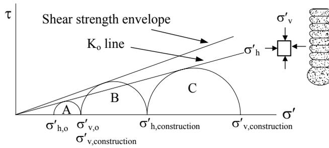
**Figure 5: Effect of increasing lateral earth pressure in decreasing settlement magnitude, after Handy, (2001).**
