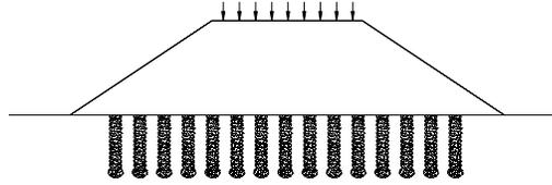
**Figure 1: Geopier reinforcement of soils beneath embankments and retaining walls**
