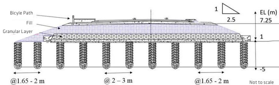
Figure 3: Typical cross section of the Impact® solution from Geopier Foundation Company
