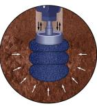
Today over 10,000 structures worldwide are supported by RAP technologies — GP3®, Impact®, Rampact®, and X1® systems. Geopier Systems are used to reinforce inadequate soils, including soft to stiff clay and silt; loose to medium dense sand; organic silt and peat; variable, uncontrolled fill; including soils below the ground water table.
