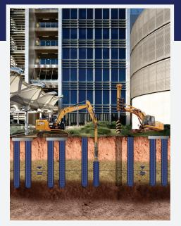
**RAMMED AGGREGATE PIER® (RAP)** Direct vertical ramming energy that provides superior support capacity, increased bearing pressure (up to 10,000 psf), and superior settlement control
