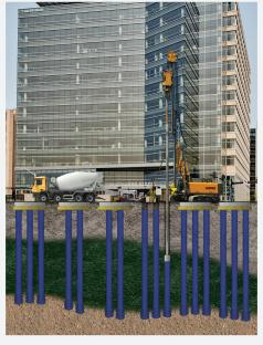
**RIGID INCLUSION (RI)** High stiffness elements constructed of cement, aggregate/grout mixture, or cement-treated aggregate
