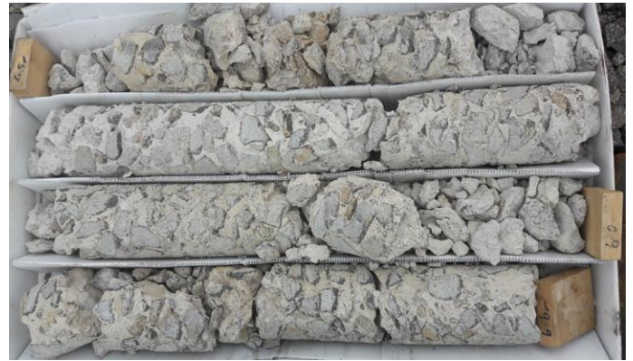
Figure 7: Grouted RAP core samples.
